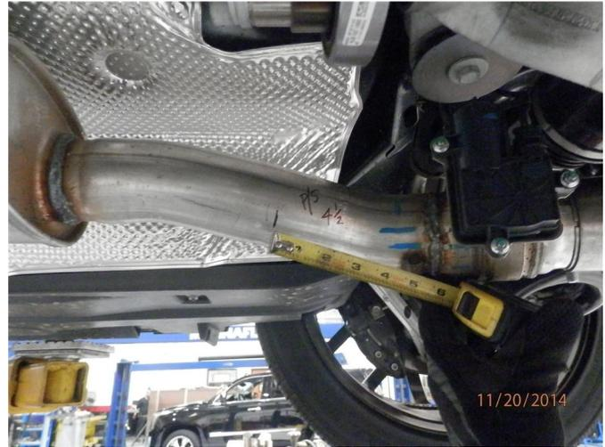
**Step 4.** For the passengers side cut 4.50" in front of the welded hanger forward of exhaust control valve as shown in the attached picture. With both valve assemblies cut from the OEM system, loosen the band clamps attaching the mufflers to the OEM tips. Both tail pipe sections may now be removed.
