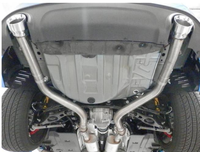
**Step 8.** Loosely attach each Tail Pipe Assembly to the Mid Pipes using the supplied clamps. Engage the welded hangers for each to the rubber insulators.
