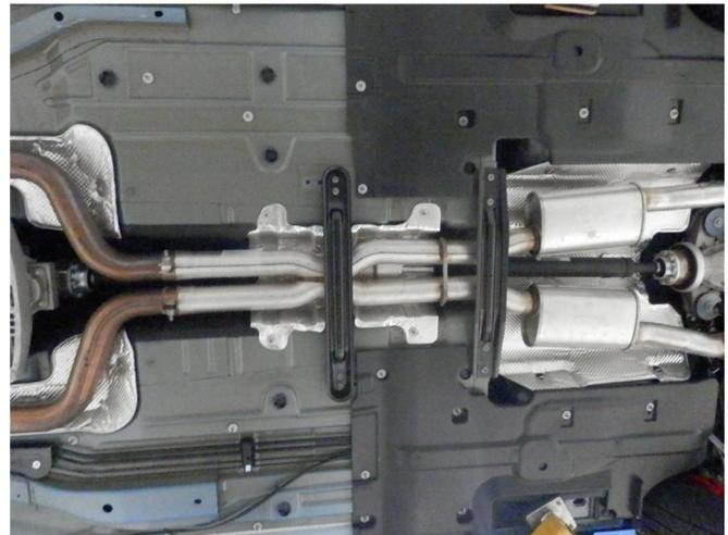
**Step 5.** Loosen the two OEM clamps at the outlet of the catalytic converters and remove the two OEM cross braces. Carefully remove the rest of the exhaust system. Disengage all welded hangers from the rubber insulators. Do not discard or damage the clamps or rubber insulators as they will be needed to install the new system.
