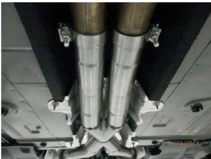
**Step 6.** Begin installation of the new system by slipping the inlet tubes corresponding with your vehicle. Loosely securing associated clamps provided. Next slip on the X-Pipe Muffler Assembly over the inlet tube adaptors. Loosely secure using two of the supplied 3.00" clamps. Orientation of the Muffler Assembly can be confirmed by the MF logo being "upright" after installation.
