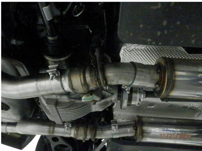
**Step 7.** Next, loosely fasten the X-Pipe Muffler Assembly outlet pipes to the OEM control valve outlet that you have just cut using the supplied 2.75" clamps. Attach the two Mid Pipes in a similar fashion to the outlet of the control valve.
