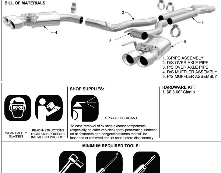
10mm, 13mm 15mm, Torx T-20 Hanger Tool (Or Pry Bar)
