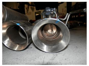
**Step 4.** Before installing your new exhasut system attach the OEM valve motors to each valve using the OEM hardware. The alignment spring on the motor will need to be engaged into the keyway slot of the new valves.
