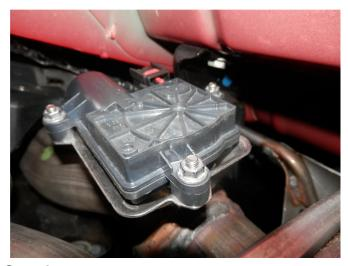
**Step 3.** Once the OEM system has been removed undo three nuts attaching each exhaust valve motor to the valve and remove. Retain the mounting hardware as it will be needed to re mount the valve motors.
