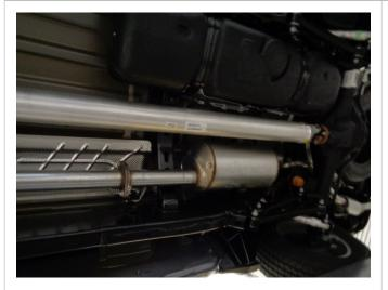
Step 1: To remove the OEM exhaust system, loosen hardware at the muffler flange.
