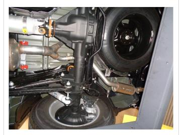
Step 2: Working front to rear disengage all welded hangers from the rubber insulators and remove the system. (Retain the insulators as they will be needed to mount the new MAGNAFLOW system.)
