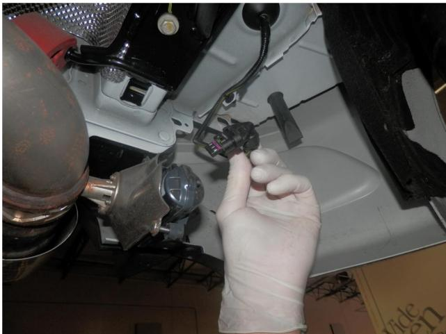
**Step 1.** Before removing the OEM exhaust first need to unplug the electrical connection on the exhaust valve control motor located on the OEM muffler assembly.
