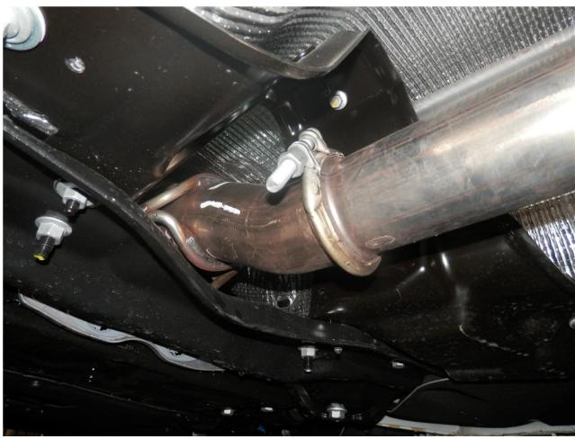
**Step 2.** To remove the OEM exhaust system begin by loosening the clamp located behind the front crossmember. Working from front to rear disengage all welded hangers from the rubber insulators. Retain all mounting hardware as it will be needed to mount your new MAGNAFLOW system.
