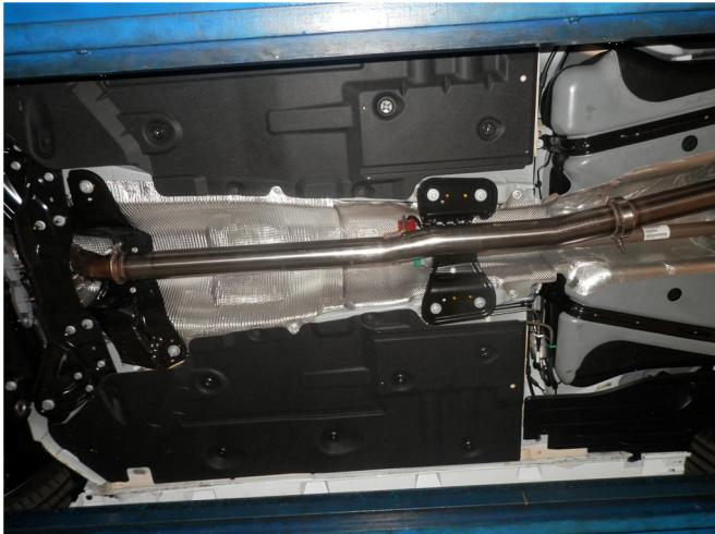
**Step 4.** Loosely Install the Inlet Pipe Assembly to the exhaust outlet using the OE clamp. Engage the welded hanger to the rubber insulator.
